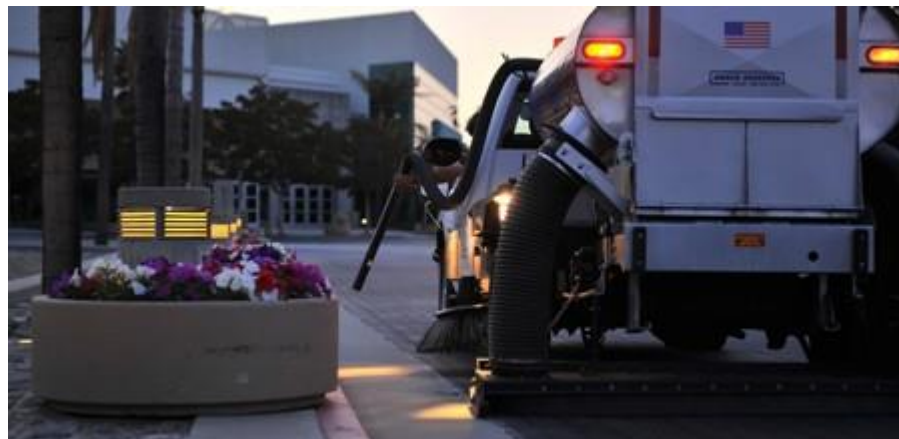
Figure 1.5: Vacuum Sweeper Service for Permeable Pavement. Source: FHWA (2000)
